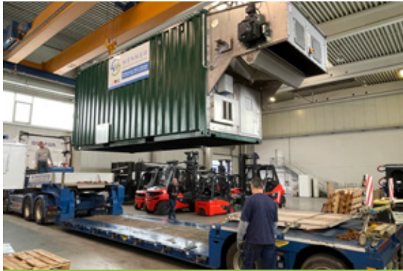
Loading of dryer module 2024 at workshop Wenner Systemtechnik
